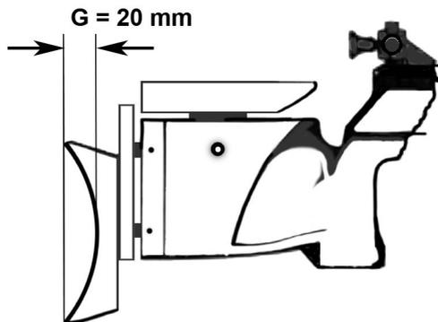
204.4.1 [G] – The curvature of the buttplate must not exceed 20 mm at its deepest point.
