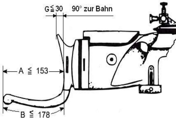
204.3.1 [A] – The distance between the outer end of the butthook on the buttplate touching the shoulder and the lowest point of the curvature of the buttplate may not exceed 153 mm. The measurement is taken from a vertical parallel to the track that touches the lowest point of the buttplate.
